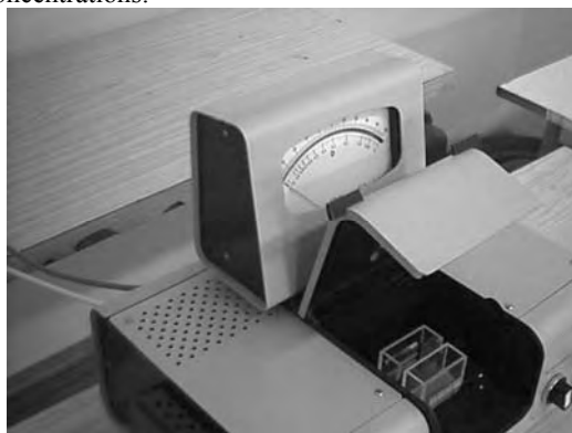
Fig. 1. General image of the electric photocolorimeter KFK – 2, including the chamber of measuring and etalon cuvettes, in working position.
