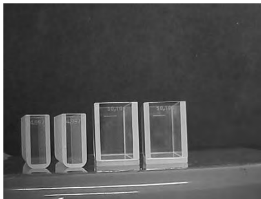
Fig. 3. Pairs of cuvettes of 50 mm optical path used in transmittance measurements based on KFK2 electric photocolorimeter (right positioned pair) and on SPECOL 10/EK5 (left positioned pair). Optical path or capacity of cuvettes may be read directly in the image.
