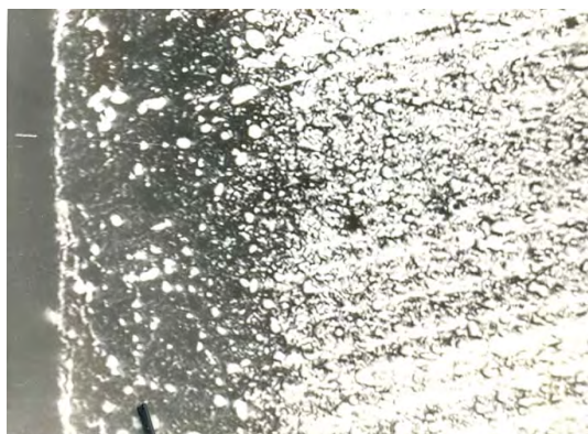
Fig. 4. Rp5 steel cyanurated 20 min at d=3,5A/m^2 , Nital attack, magnify: 700:1.
