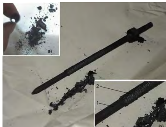
Figure 9. Pyrolysis graphite layer resulted from thermal destruction of polystyrene: a) aspect of the pyrolysis graphite layer resulted from thermal destruction of polystyrene; b) aspect of the deposit of pyrolysis graphite on holde; 1- holder for pyrolysis graphite collection; 2- aspect of the pyrolysis graphite deposit
