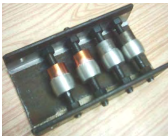
Fig. 7. The compression device for the welded samples and the electrical furnace.
