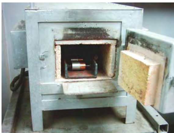
Fig. 7. The compression device for the welded samples and the electrical furnace.
